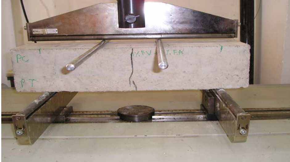
Figure III.4. Mode de rupture ductile
