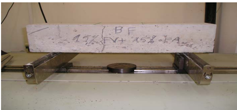
Figure III.5. Densification de fissures et rupture ductile
