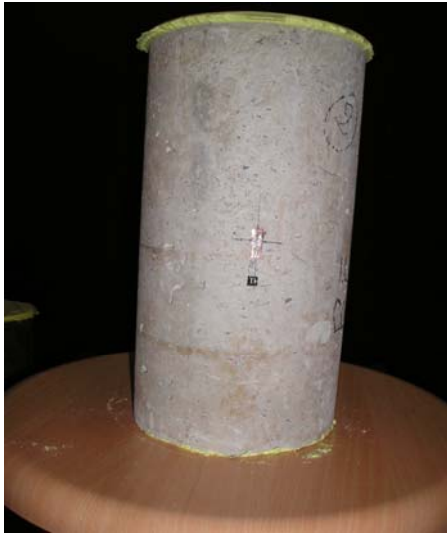
Figure III.11.a. Rectification des faces
