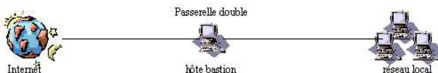
Figure 26 : La passerelle double.
