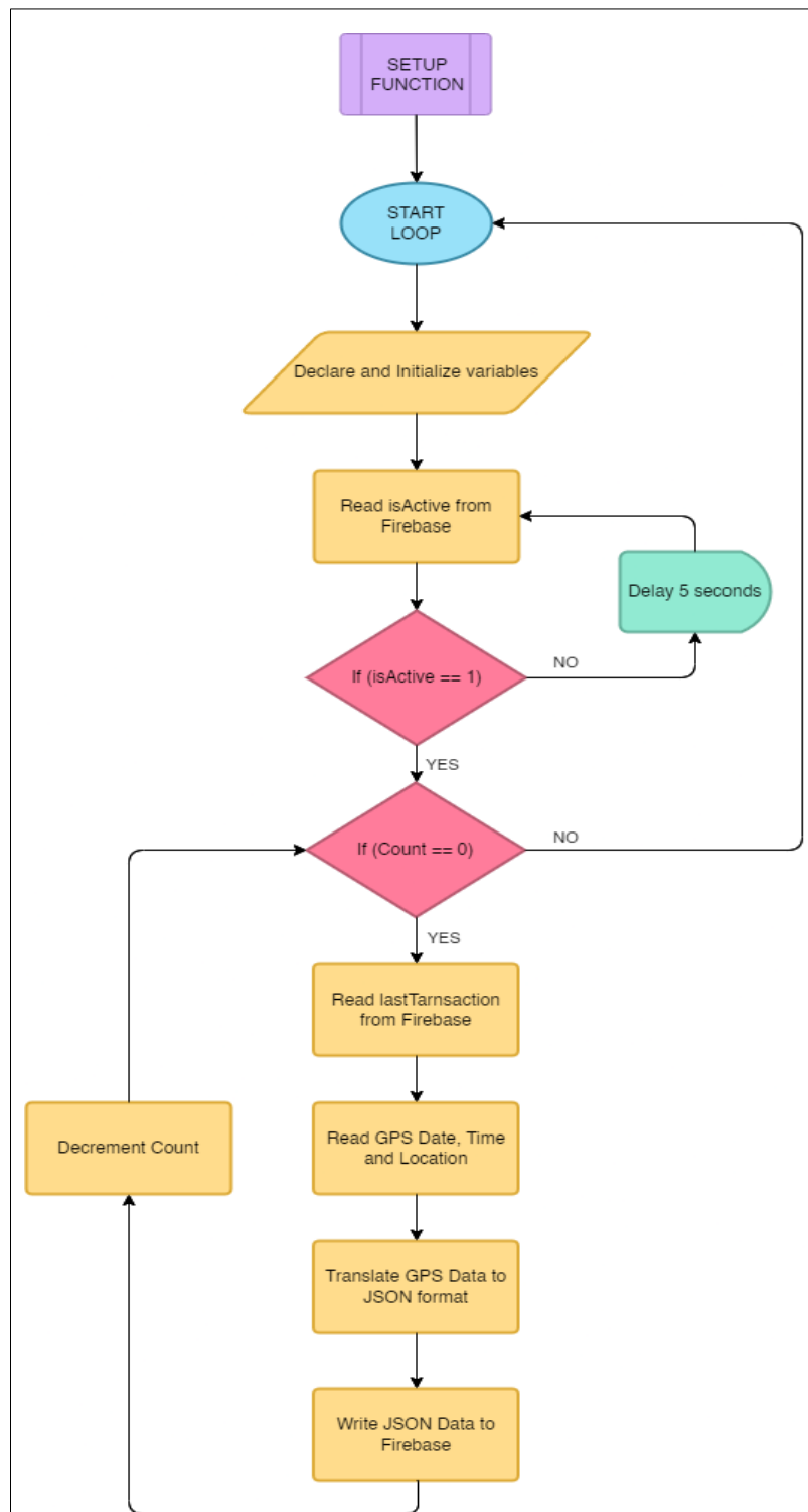
Figure 43 Arduino Loop Function Flowchart
