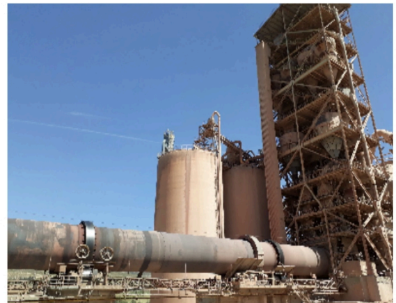
(b) cooler system with its heat ex-changer and to the left and kiln appears to the right
