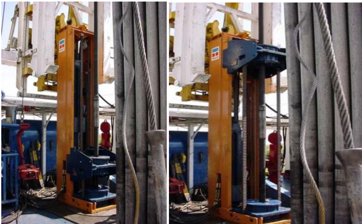
Figure III.12 : Unité Push-Pull Rig Assist (Courtesy Tesco)
