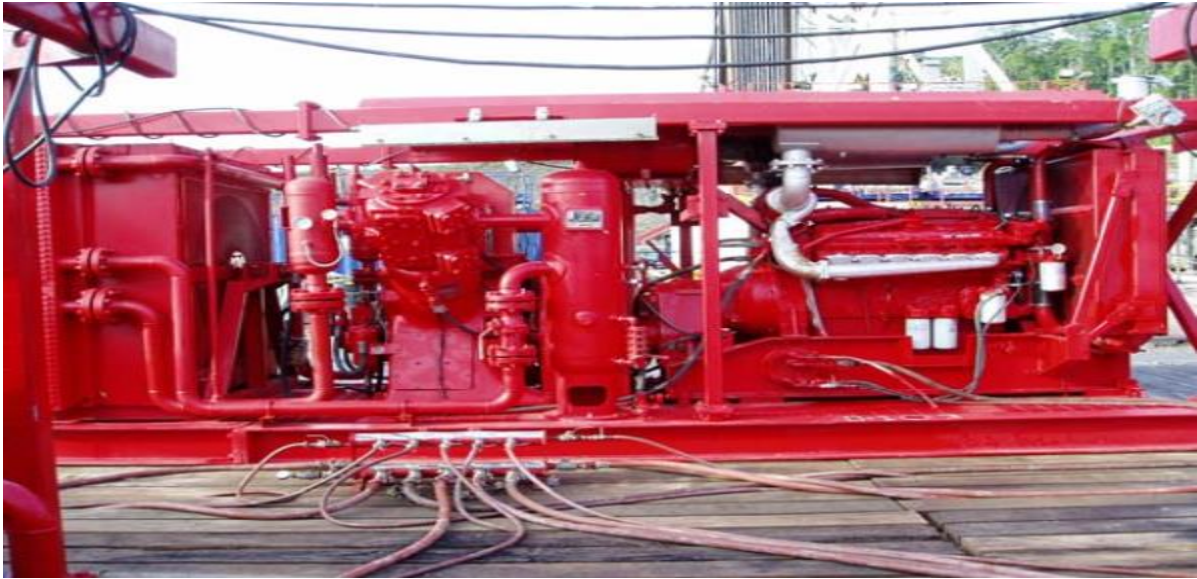
Figure III.5 : WB-12 Low Pressure Booster (1800psi)
