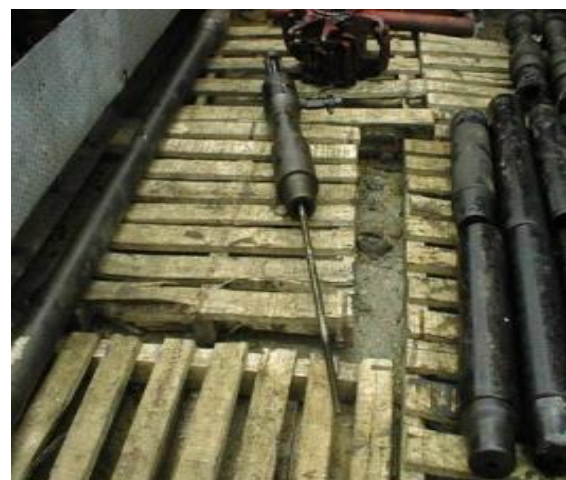
Figure III.27 : la NRV (non return valve)
