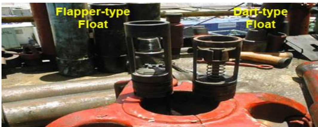
Figure III.26 : Les types de Flapper anti-retour
