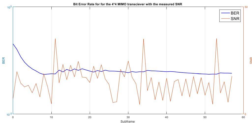
Figure 3. 21:Bit Error Rate for the 4*4 MIMO transceiver the measured SNR for each subframe
