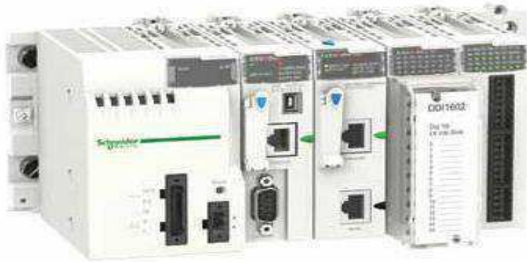
Figure III.2 : Automate programmable industriel. Type Schneider
