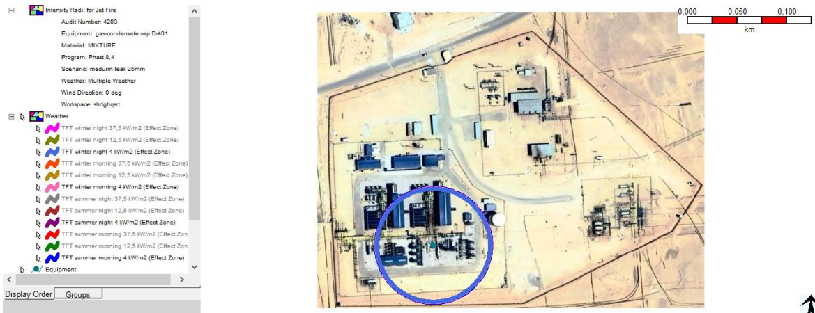
Figure 3-3 Flammable gas cloud footprint for a medium leak scenario
