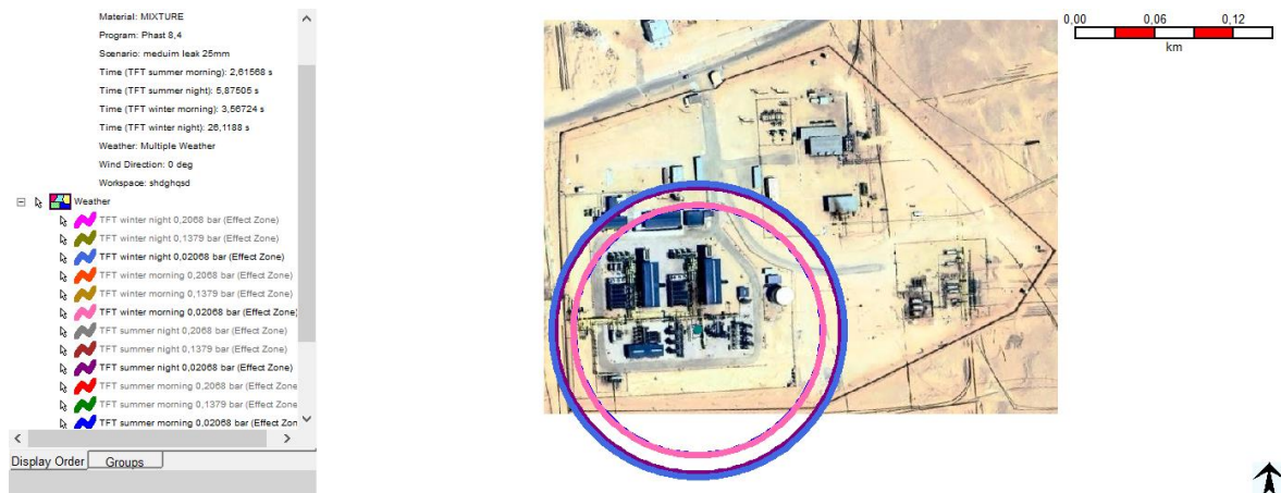
Figure 3-6 Explosion overpressure contours for the worst-case scenario
