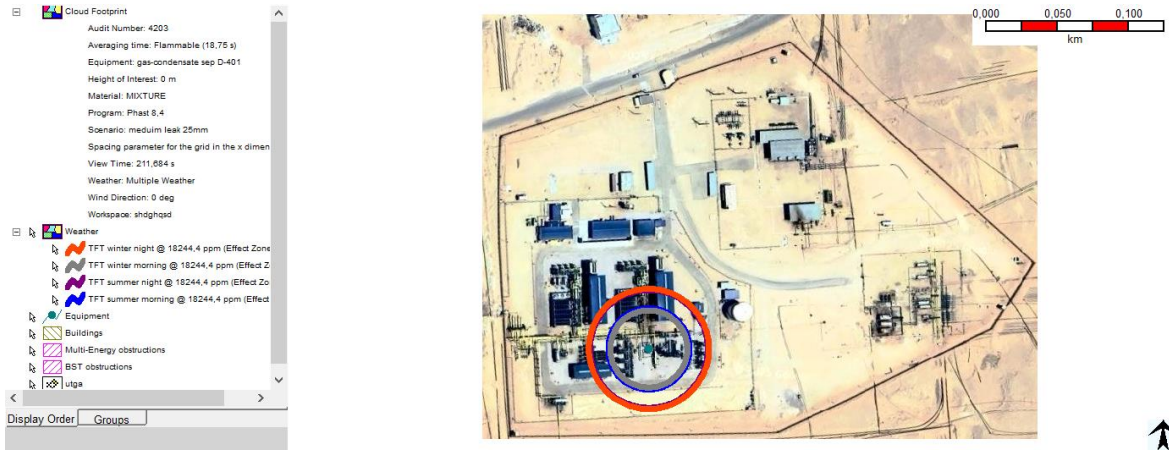
Figure 3-3 Flammable gas cloud footprint for a medium leak scenario
