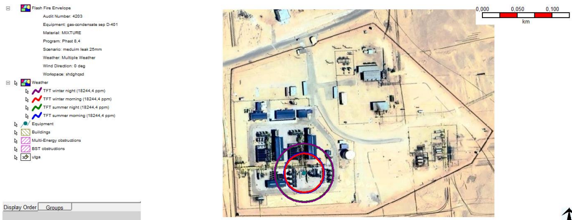
Figure 3-5 Flash fire envelope for a medium leak scenario
