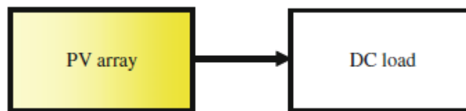
Figure 1.2: Direct-Coupled PV System. [4]
