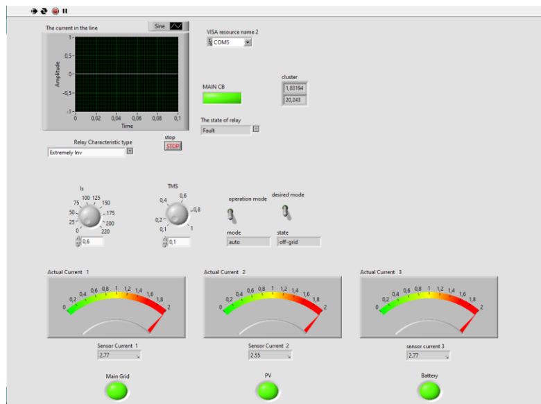
Fig 4.7: Result of General Fault
