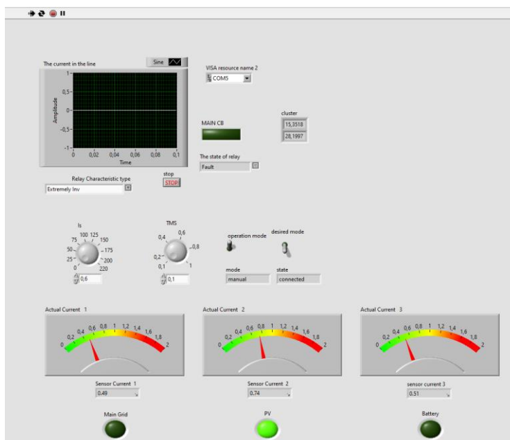
Fig 4.8: Result of Fault at PV
