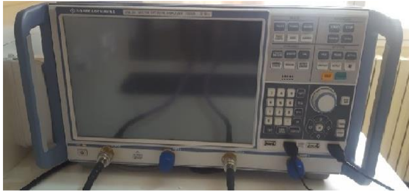
Figure 3.12 Vector network analyzer used for S_{11} measurement
