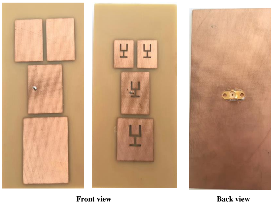
Figure 3.11 Front and back views of the realized Yagi-Uda antennas with and without slots
