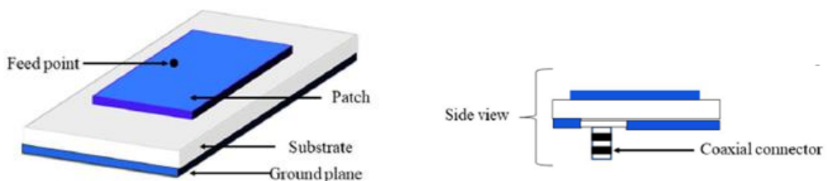
Figure 1.5 Probe feed of microstrip antenna and its side view [9]
