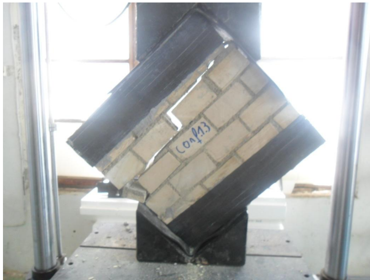
Figure IV.12: mode de rupture de CONF1.3
