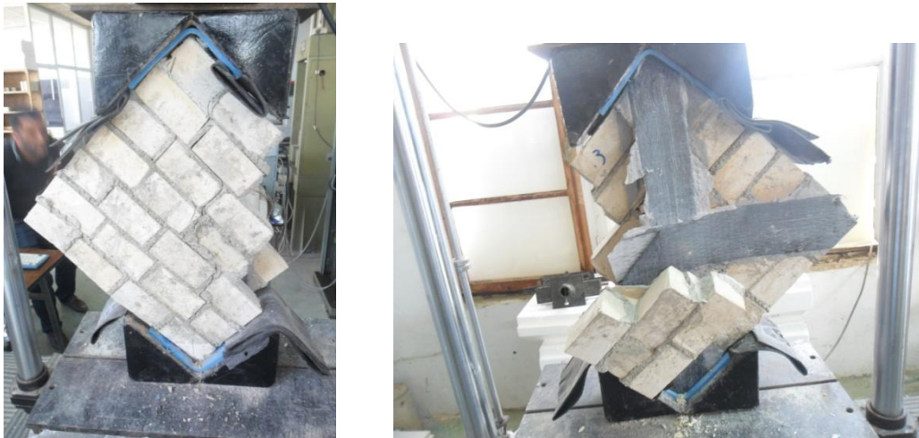
Figure IV.27: mode rupture CONF4.3
