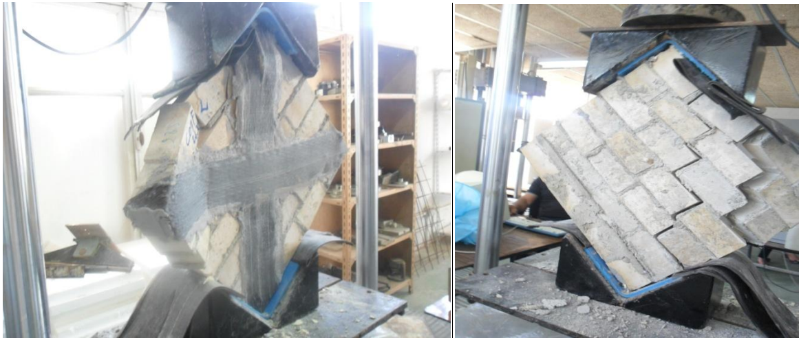
Figure IV.25: mode de rupture CONF4.2
