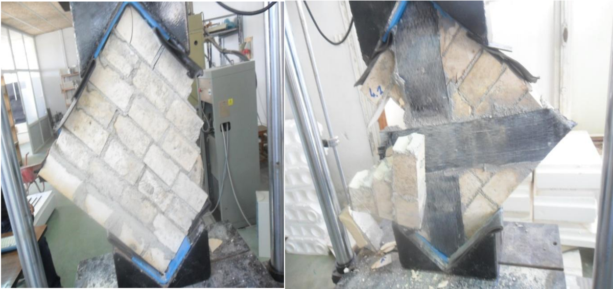
Figure IV.23 : mode de rupture CONF4.1
