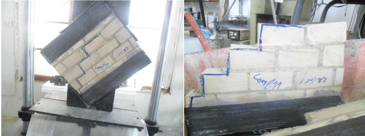
Figure IV.10: mode de rupture de CONF1.1
