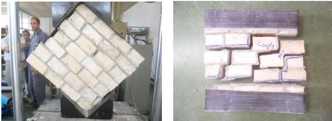
Figure IV.11: mode de rupture de CONF1.2
