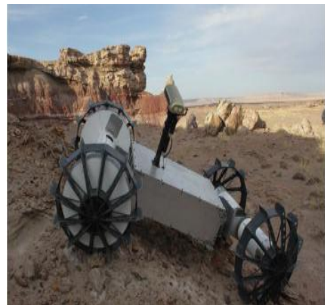
Fig 1.2: The DuAxel rover on rough terrain. DuAxel consists of two Axel-class rovers docked with a central module.
