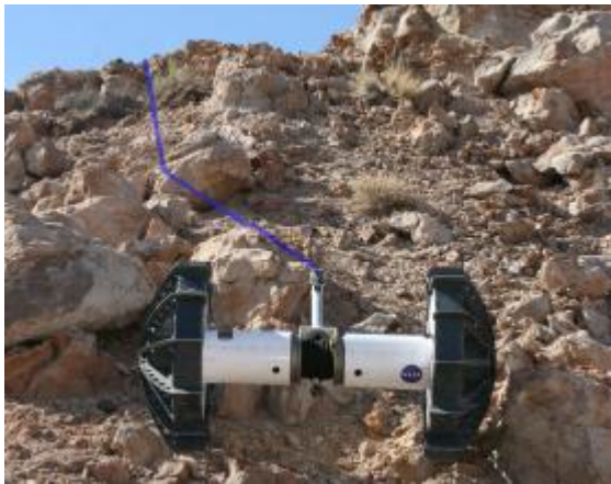
Fig. 1.1: A picture of Axel descending steep, rough terrain in Arizona desert. Tether highlighted in blue.
