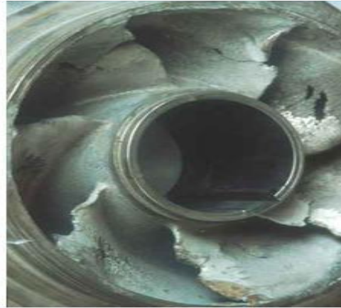
Figure I.6. Example of erosion in a material.
