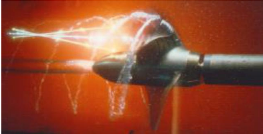
Figure I.5. Illustration of vortex cavitation.
