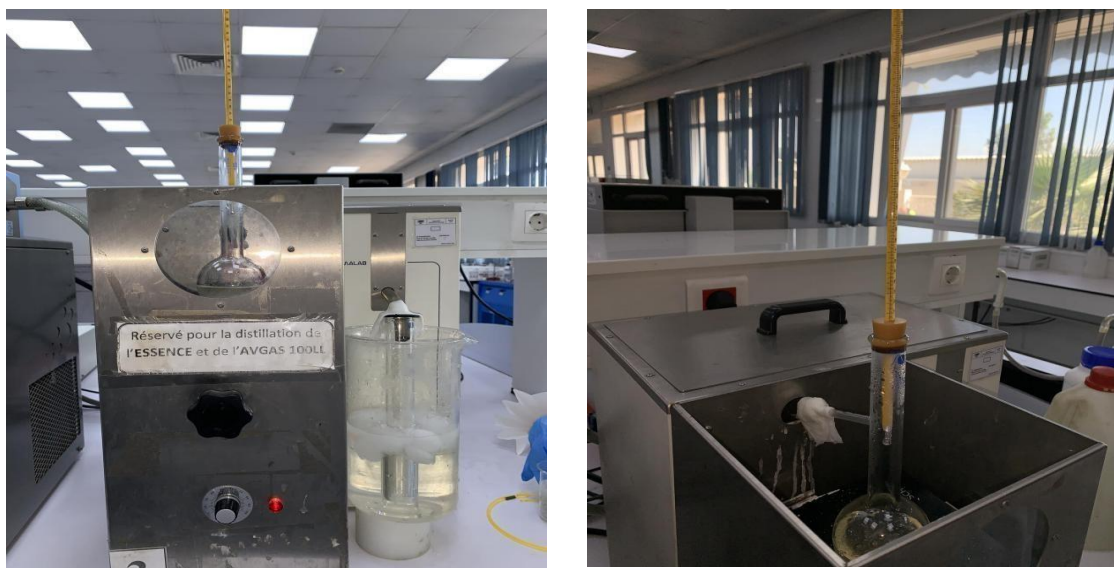
Figure II.15 : Distillation Atmosphérique ASTM D86
