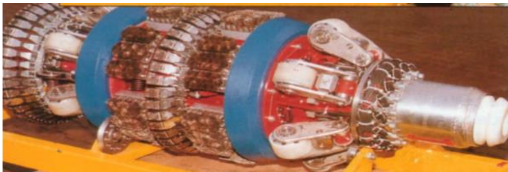
Figure II.5 : Outil intelligent de type MFL
