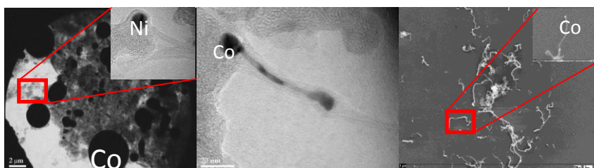
Fig. 1. Three different forms of cobalt: a) cobalt nanowires ( in-situ filling), b) spherical particle cobalt (ex-situ filling), c) cobalt nanoparticles on the top of CNTs (PECVD).
