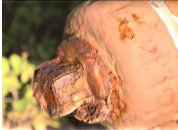
Figure II.5- La corrosion intergranulaire [3]
