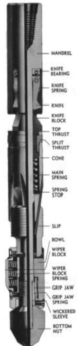
Figure 2: Internal Cutter
