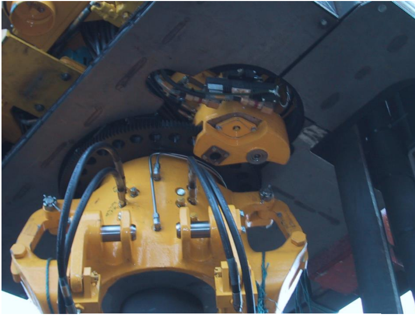
Figure A.4: Shot pin of Link Adapter
