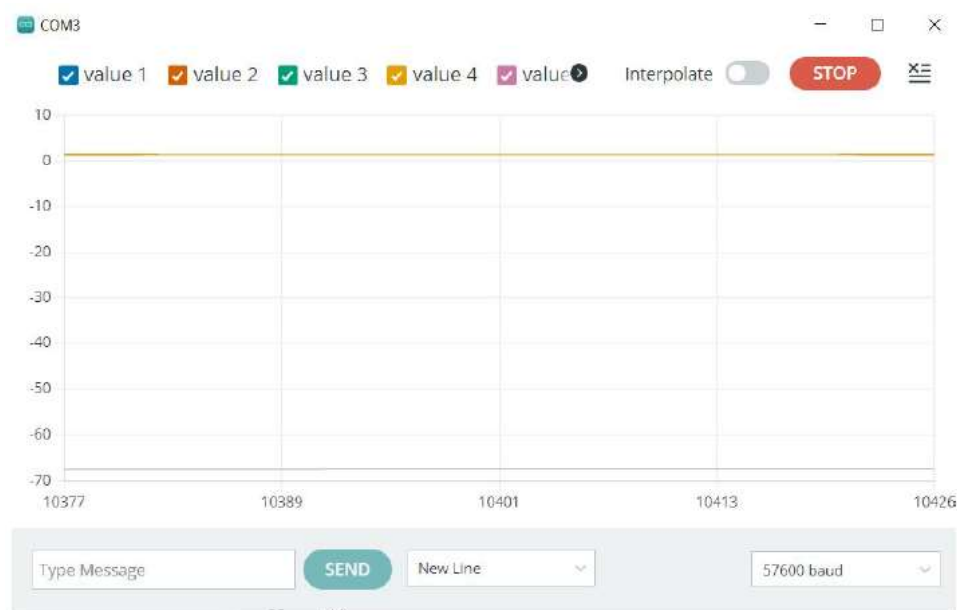
Fig. 12 MPU 6050 Data Reading after using Kalman filter.
