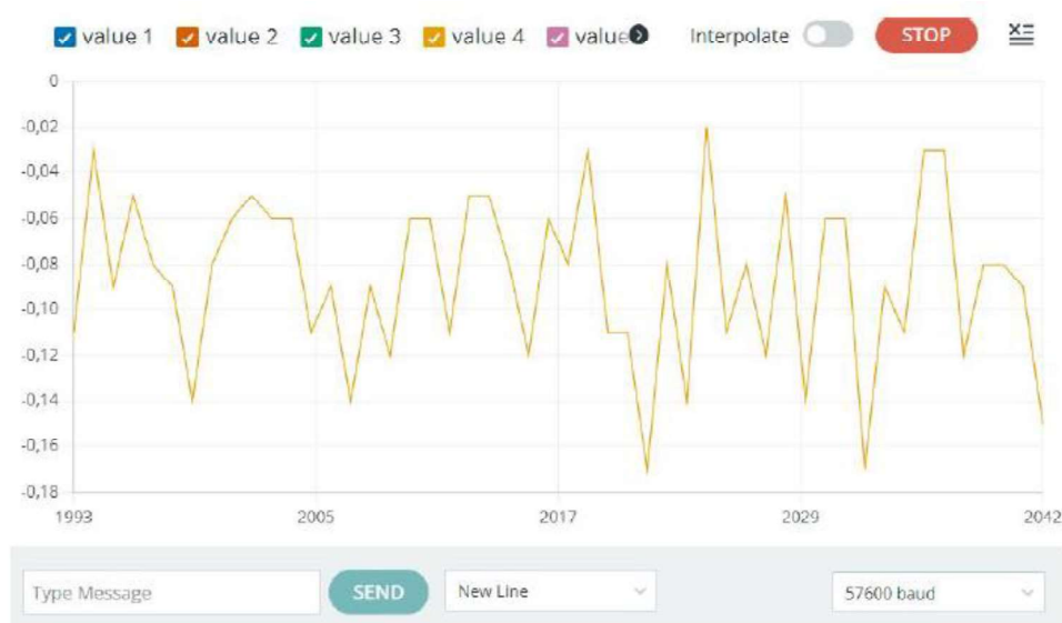
Fig. 11 MPU 6050 Data Reading before using Kalman filter.
