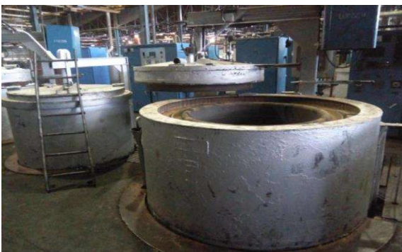
Four de cimentation
