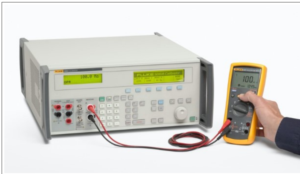
Figure 1: Calibrating a digital multimeter using reference calibrator [10].
