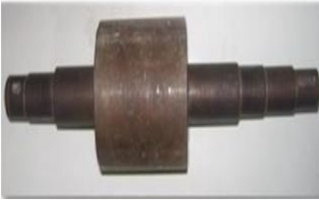
Figure II 5: Rotor massif rainuré
