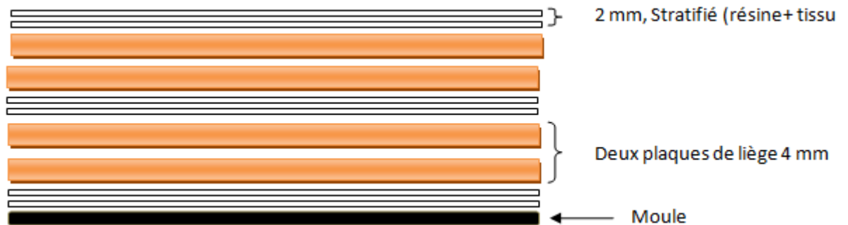
Figure III.11. Superposition de Sandwich (SDW3).
