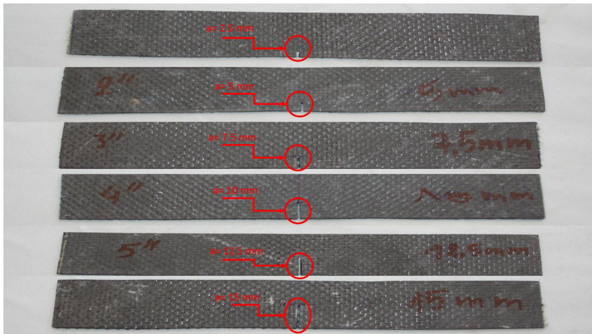
Figure. III.21 carbon/epoxy specimens with different crack sizes
