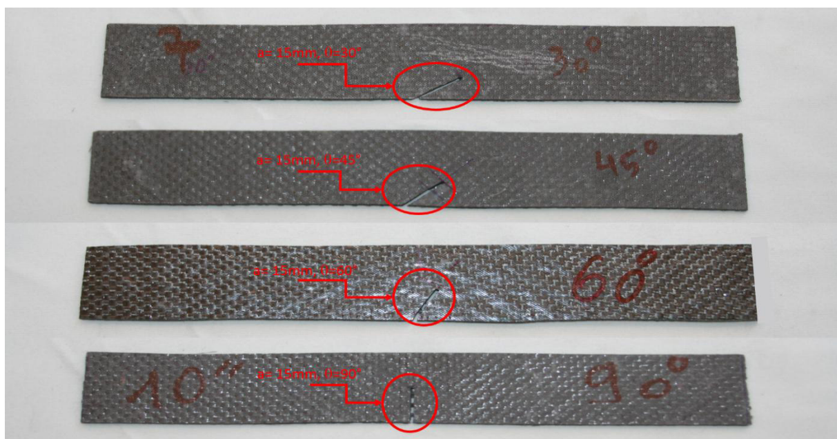
Figure. III.22 carbon/ epoxy specimens with different crack angles
