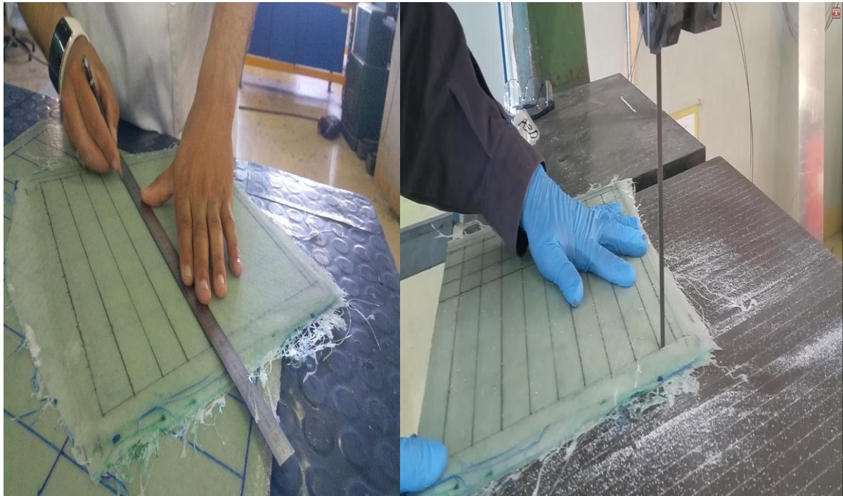
Figure. III.17 tracing and cutting the obtained composite material
