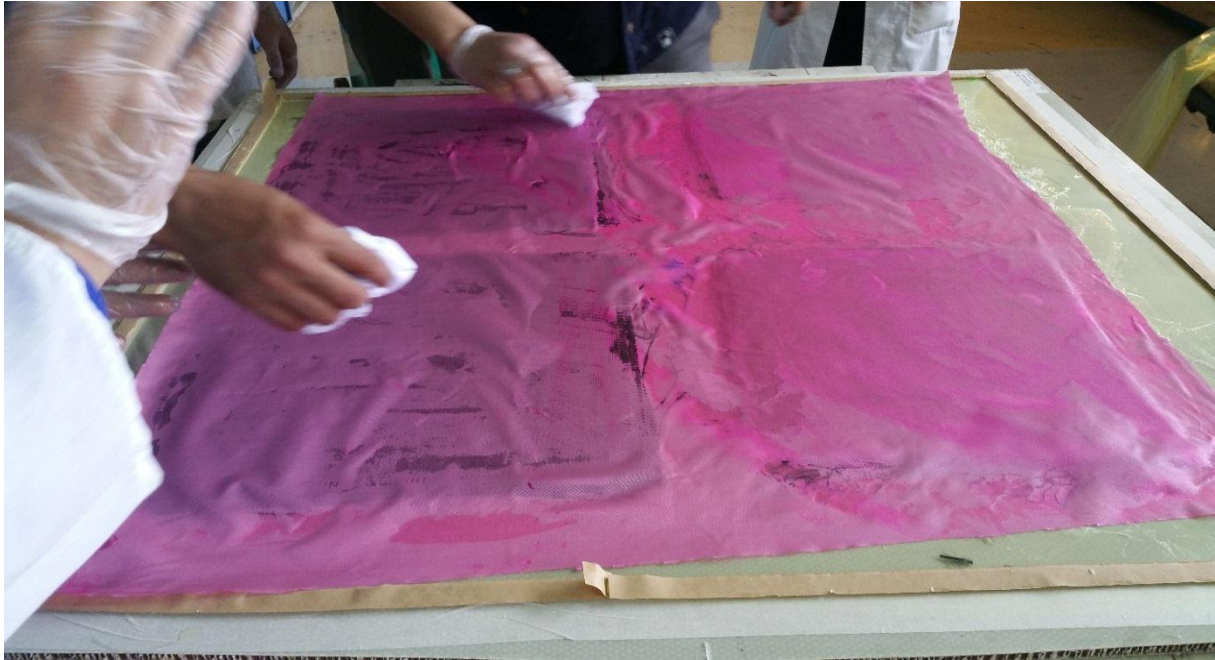
Figure. III.13 use peeling film to absorb resin
