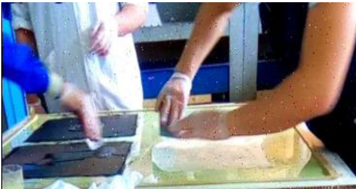
Figure. III.12 molding resin on plies
