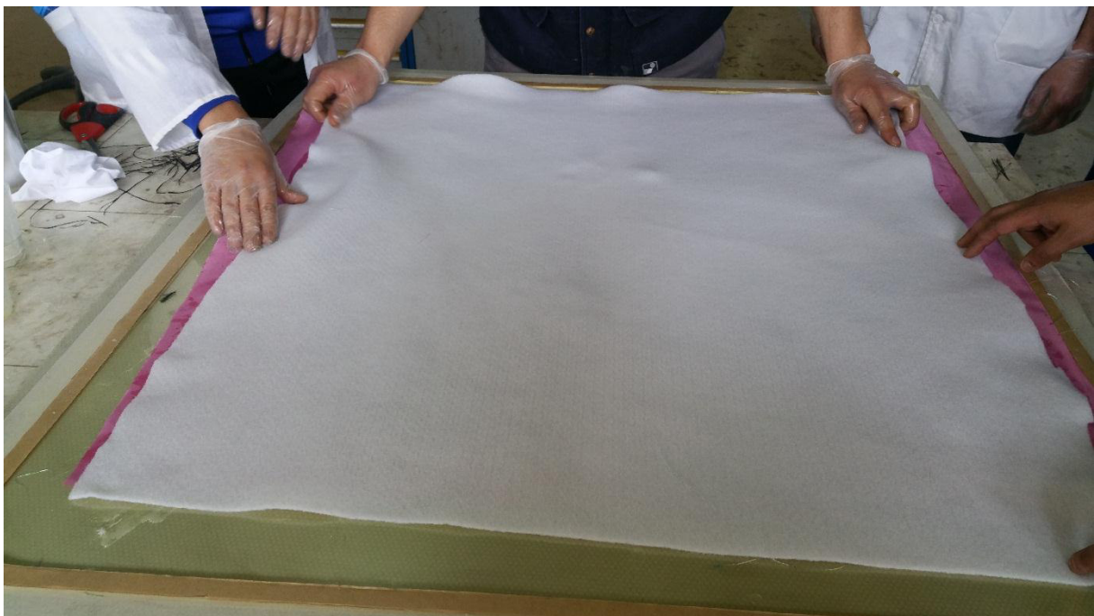
Figure. III.14 use the pumping felt to increase heat and pressure
