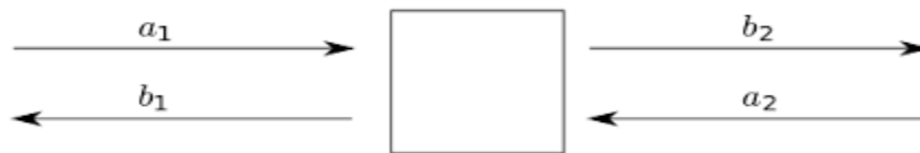
Figure 1-5 S-parameters two ports network
