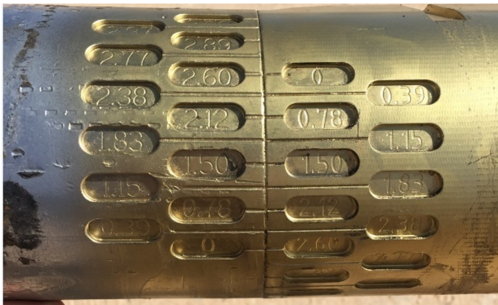
Fig(IV-6): Ajustement du Bent Housing
