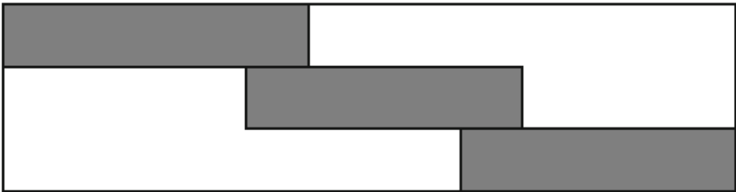
Fig.2.4. Structure of gain matrix K [33].
