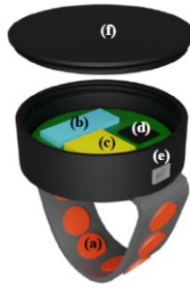
Figure 2: Exploded view of our haptic bracelet (some colors are changed for better view). Tactor (a). Communication module (b). Battery (c). STM32 micro-controller (d). charger plugin (e). Cover (f).
