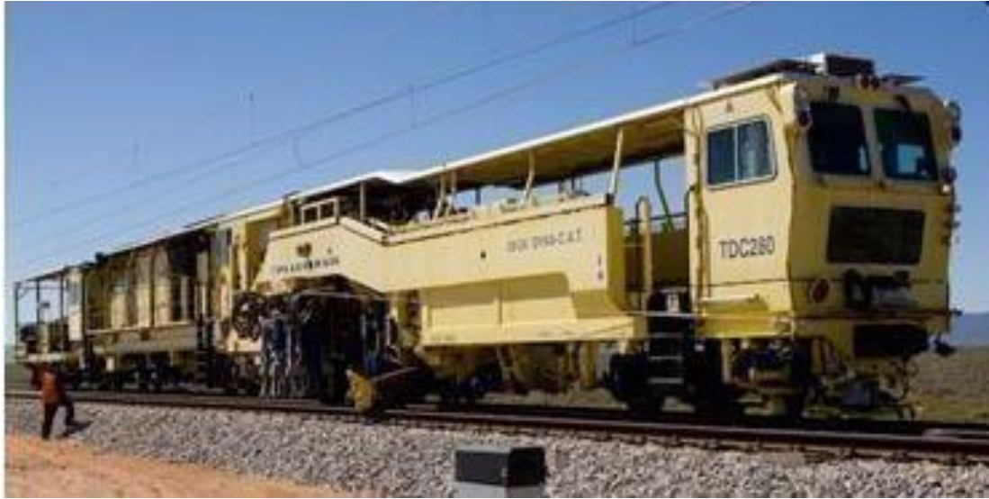
Figure III.8 : Bourreuse universelle DYNA-CAT, [1].
