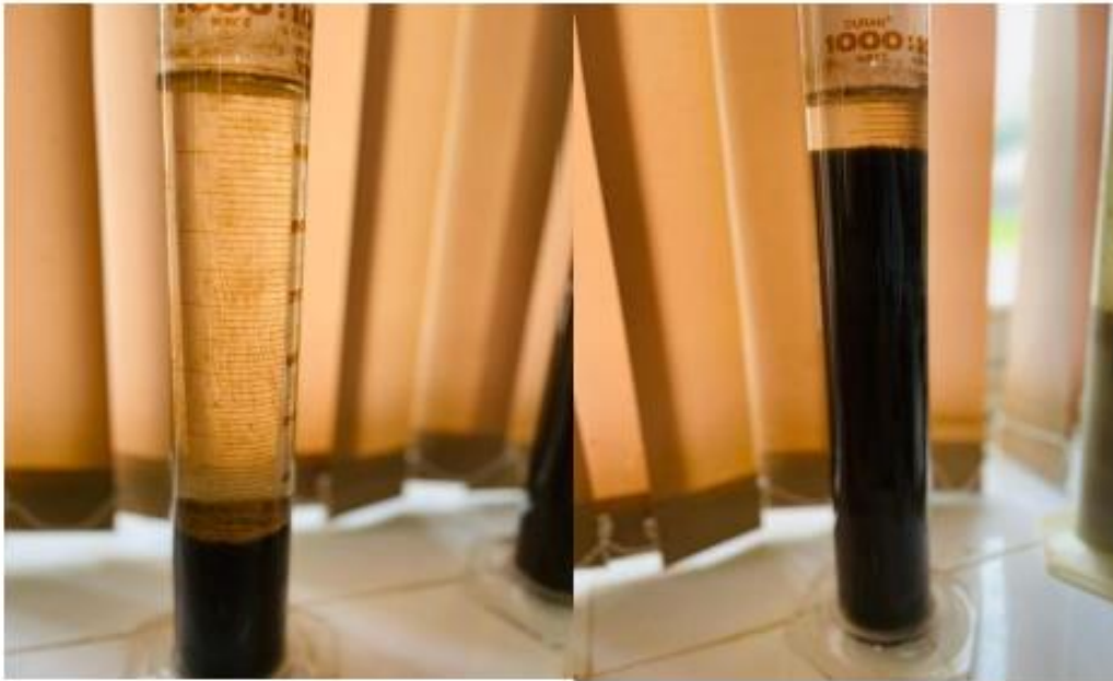
Settling of activated sludge. Settling of recycled sludge.
