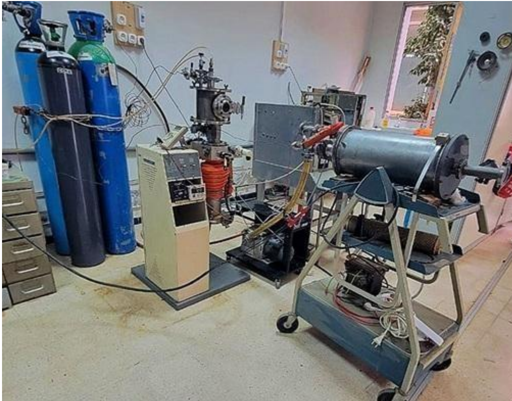
Figure 3.4. Nitriding system by ion implantation of CDTA
