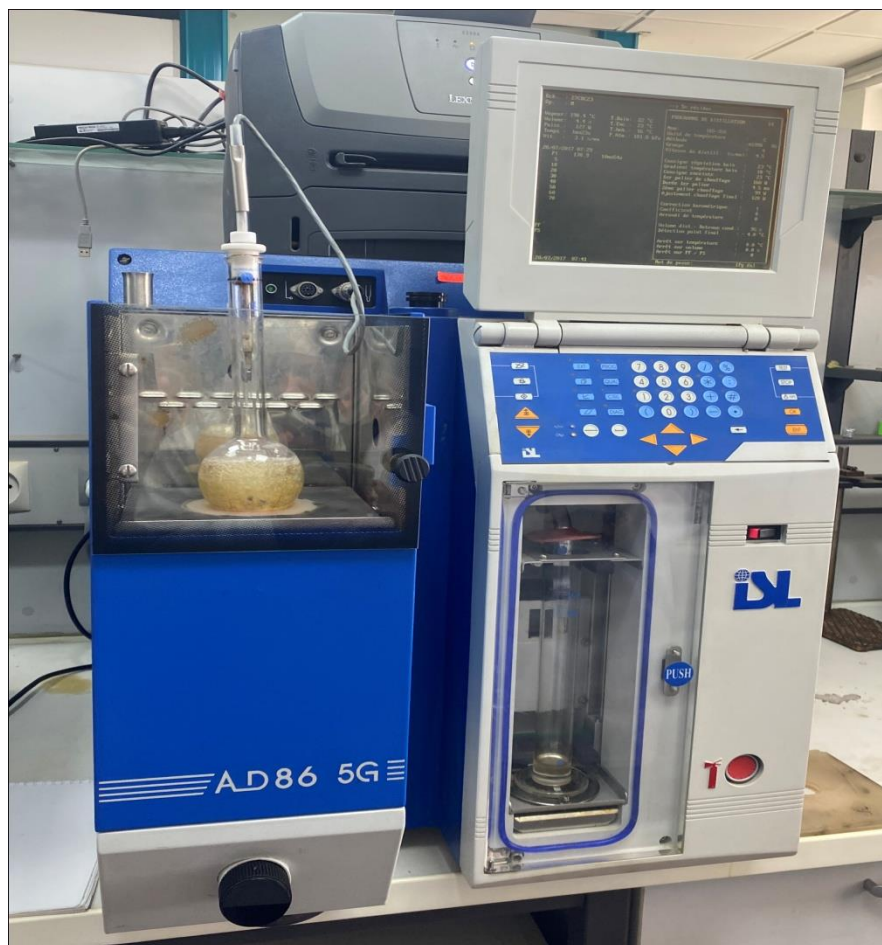
Figure IV. 17: Appareil de distillation ASTM D86.
