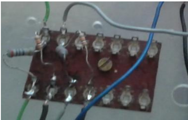
Figure IV.40 Carte injection signaux gache (MOSFET)
