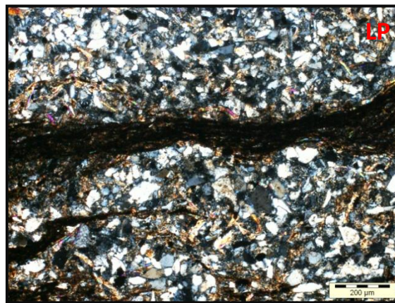
FIG.III.22: puits HNEP-1 côte 4992.52; laminations argileuse
