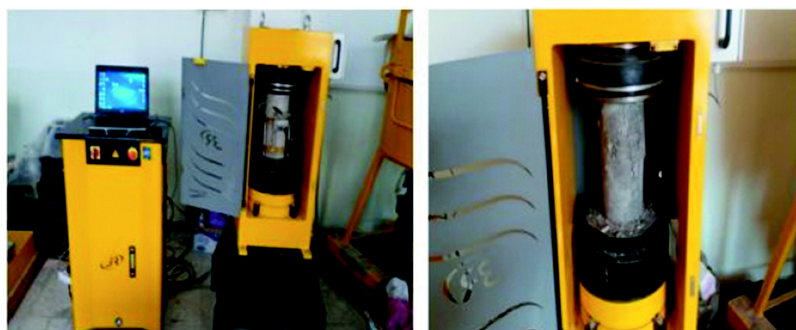
Figure 2. Compressive, extensometer apparatus (3R).
