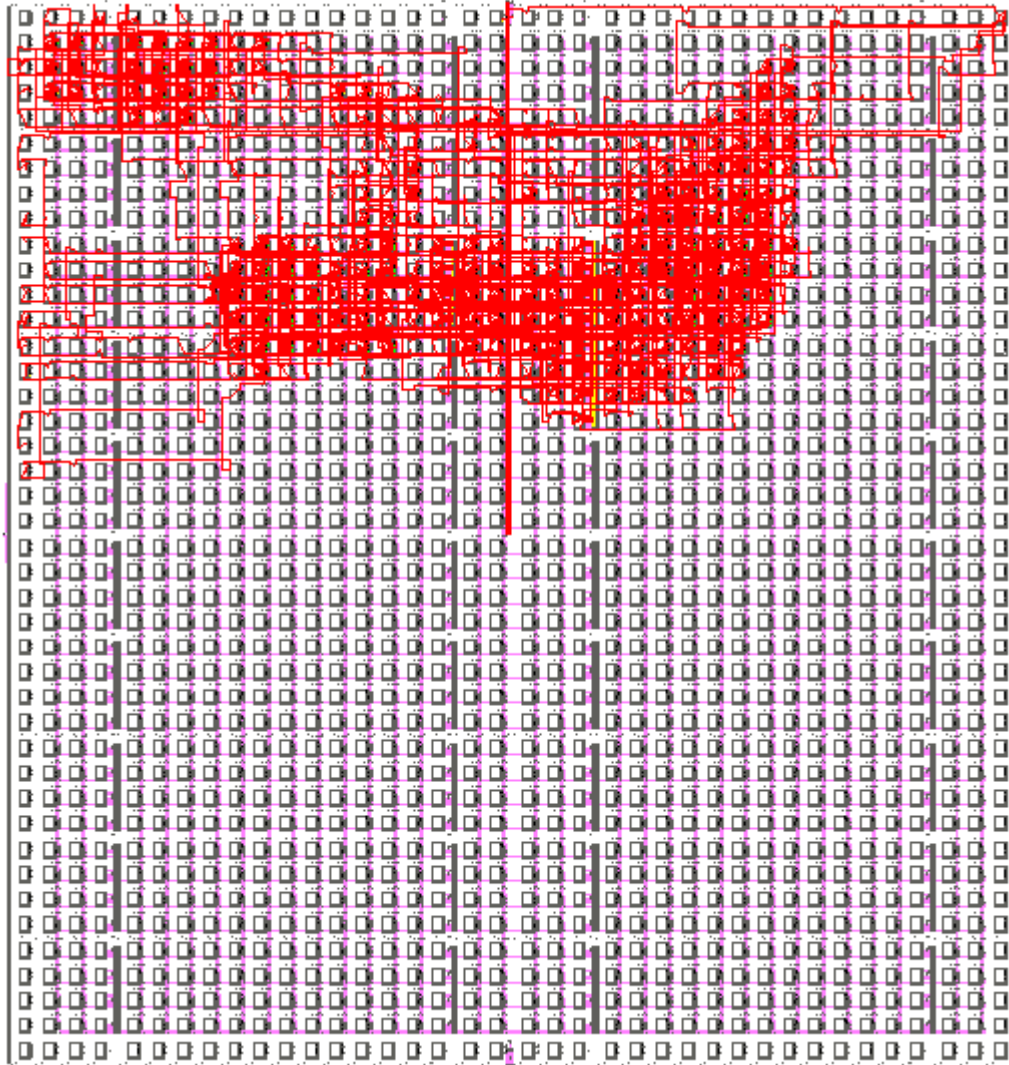
FIG5.9: Routing scheme for 16 bit interleaved multiplier created by FPGA Editor
