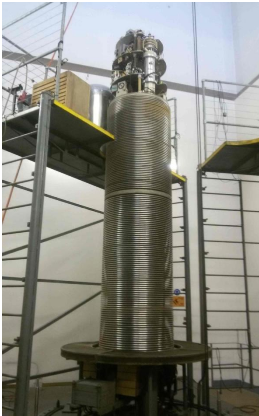
Fig. A.1: Photogeneral view of the 6MV VDG at MRD iThemba LABS.
