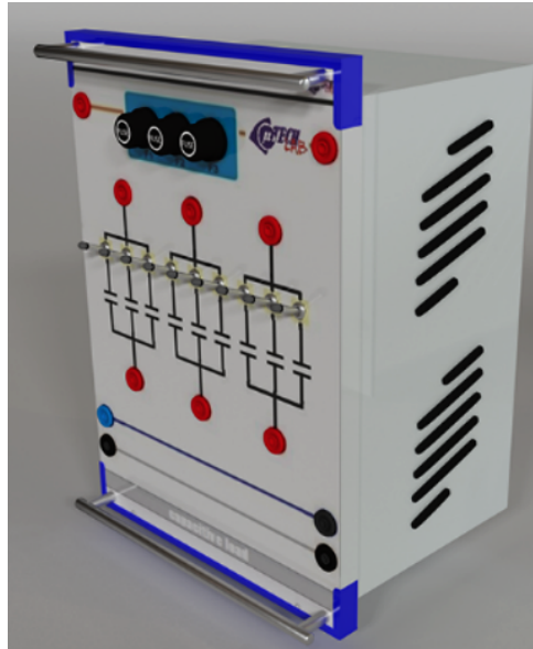
Fig. 2.4: ELE-CAP : Three phase capacitive load
