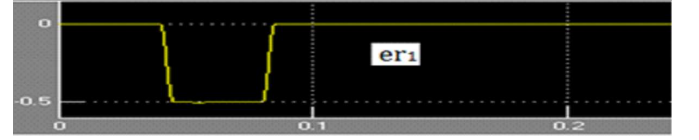
Fig. 4. Error signals for a 0.5 per unit (pu) voltage sag on phase A .
