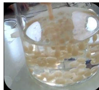
Figure 4. Formation of alginate / pectinolytic enzyme beads.
