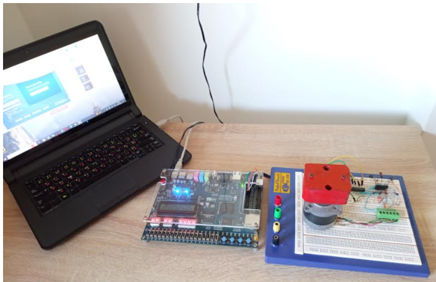
FIG. II.16 : Experimental setup : step motor on project board, driver in the right and the DE2 board in the right of PC controller interface which is seen in the left.
