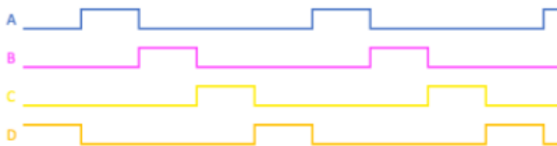
FIG. I.13 : wave drive or single coil excitation.
