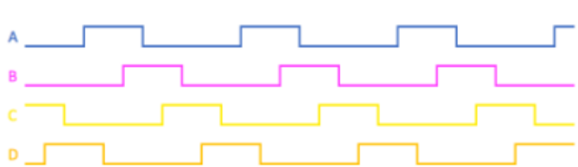
FIG. I.17 : Excitation sequence waveform of half step excitation.
