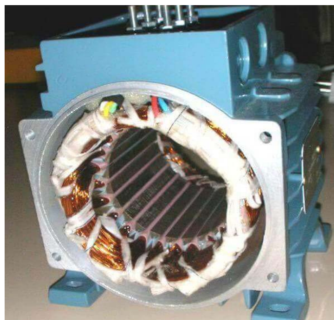
Figure II.2: Stator d'une machine asynchrone triphasé
