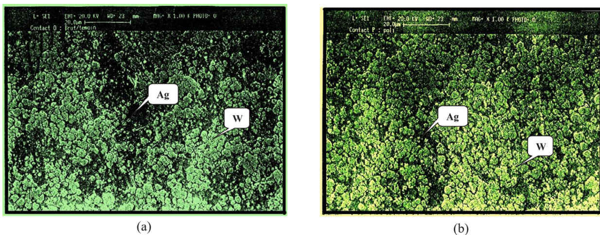
Figure 3: Micrographs for (a) a virgin contact, Ag–W (50/50) and for (b) a vacuum heated contact, Ag–W(50/50). SEM magnification \times 1000 .
